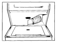
The washer lid can now be **opene**d enough to allow you to remove the agitator, and the dryer exhaust ducting is accessible for inspection and cleaning.
